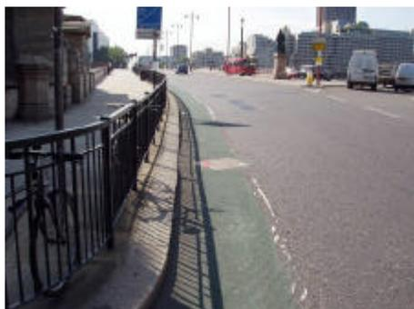
The east side bus stop is dangerous to cyclists because they will be “clipped” trying to cycle around the stopped bus. Cars go fast here if the light is green at the pedestrian crossing. At this place there is only one drive lane, but cars may squeeze towards the left-turn lane and outer through-lane in relation to the junction at Stamford Street.
