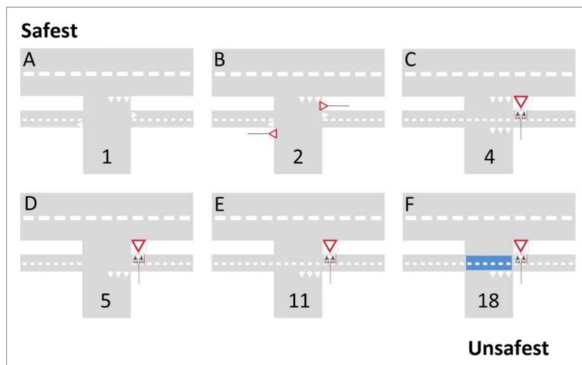
Figure 3 presents in an easy understandable way the accident prediction model based on the 332 sites that have remained unchanged for the period 2000-2011. Design F has about 18 times more bicycle and moped accidents than design A when traffic volumes on the path and the nearby intersection/roundabout are the same.
