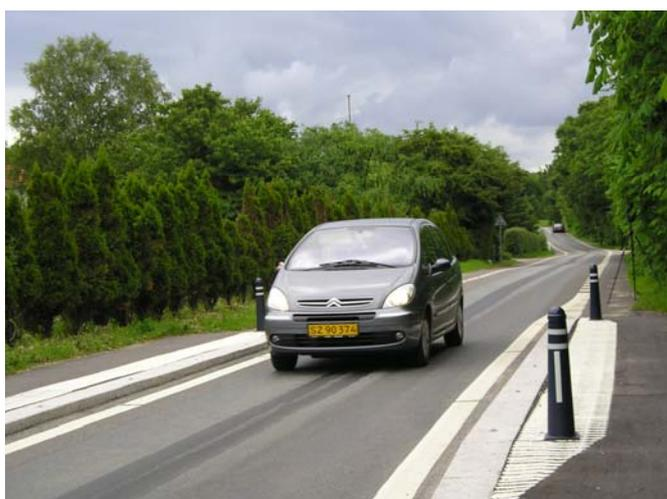
Figure 6.2: Speed reducer designed as narrowing with only one central vehicle lane
