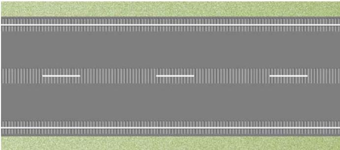
Figure 4.4: Rumble road surface along centre line and edge lines
