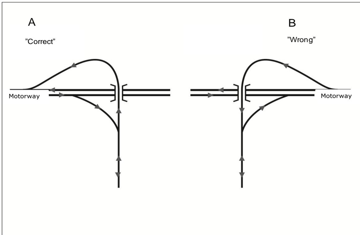
**FIGURE 2: Two design principles A) and B) for “half-intersections” between motorway and two-lane rural road. Design B) might mislead the driver to choose the wrong ramp. You should never have a “straight ahead” road “inviting” you if you are not allowed to enter.**
