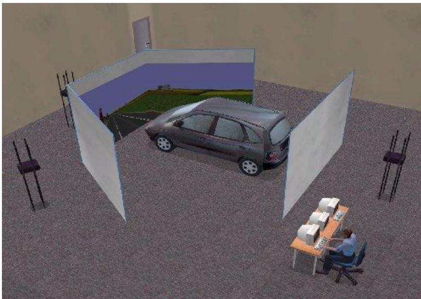
**FIGURE 1** Vehicle simulator. The field of view makes it possible for test drivers to see the road from the windscreen, rear-view mirror and side-view mirror, and in an angle of 45 degrees to each side.
