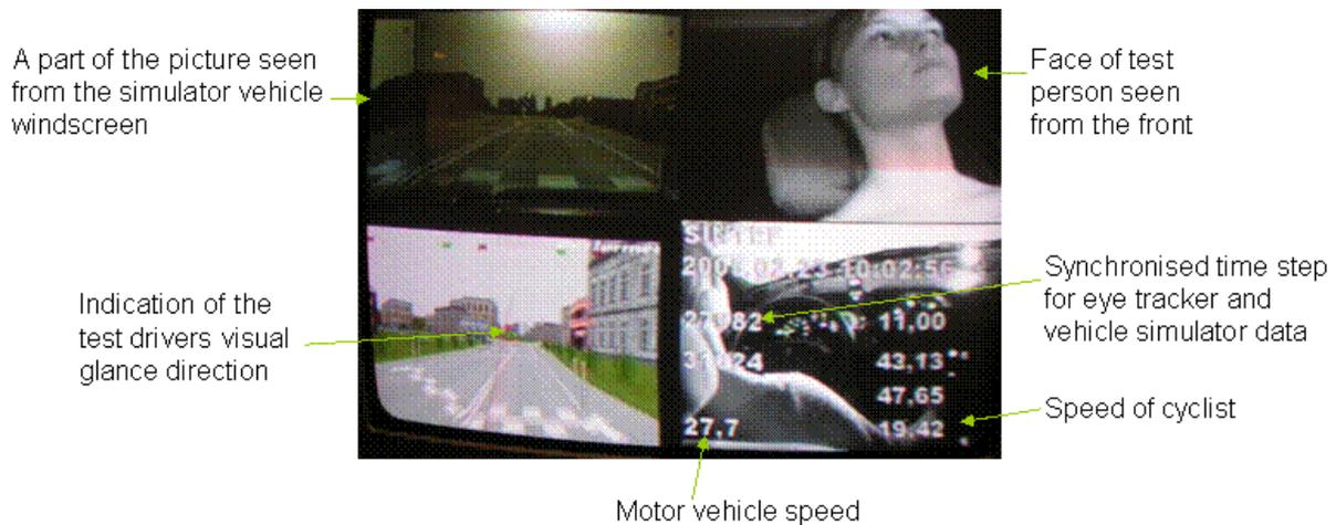
**FIGURE 2 Example of video recording of test drive. The four pictures are synchronised.**
