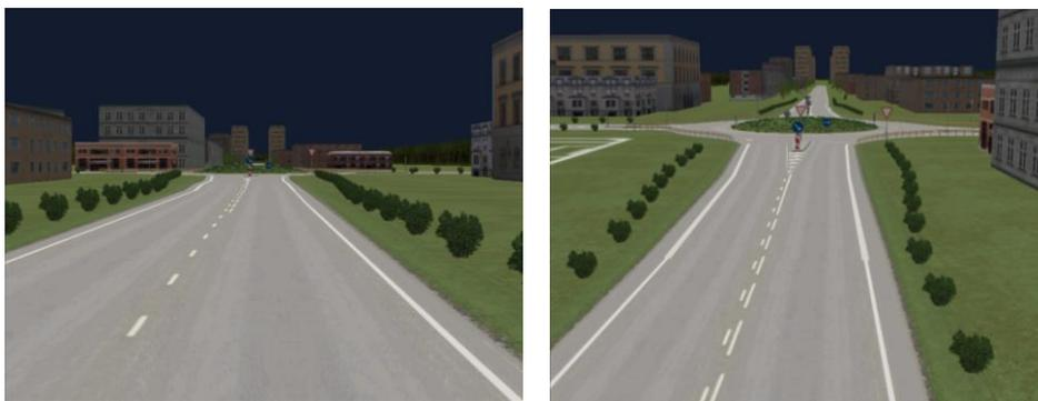
Example of roundabout with medium visibility splays. Height of the central island is 1.5m with the plantation included. Height of bushes on the approach are 0.8 m.
