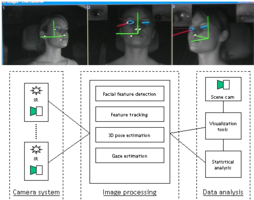
**FIGURE 4** Process sketch of the eye tracker. By identifying a number of land markings on the test driver's face (here eyes, mouth corner, nostrils and earlobes) and matching these to points in the 3D computation of the driver's head, a calculation of the orientation and positioning of the subjects eye can be made with great precision. The 3D model can then place the eye's iris and pupil again and determine the direction of the gaze.
