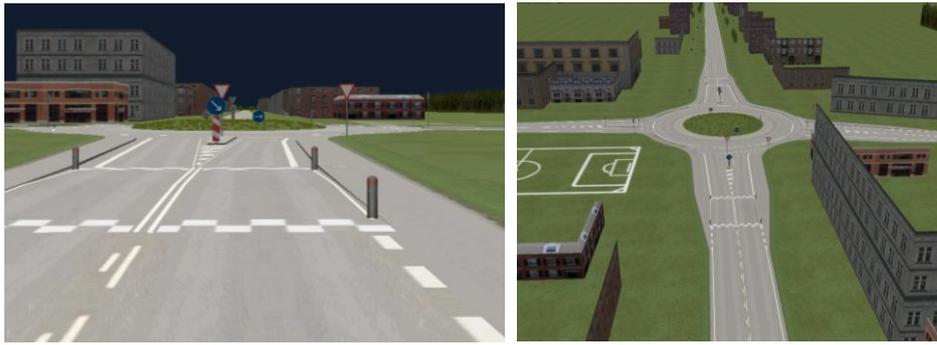
Example of roundabout with good visibility splays. No plantation in the approach. Height of the central island is 1.0 m with the plantation included.
