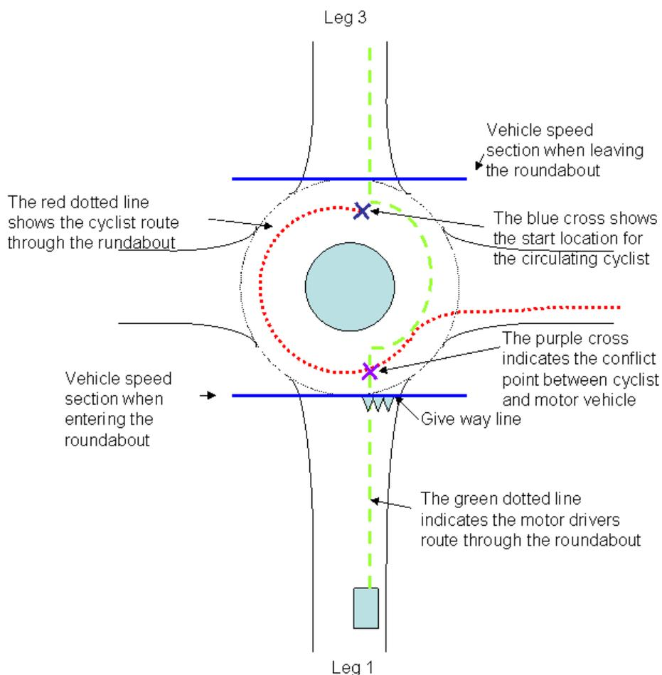
**FIGURE 7** The Observation area starts 150 meters before the give way line (leg 1) and continues up to the point where the test driver leaves the roundabout (leg 3). The purple cross indicates the conflict point between the circulating cyclist and the entering motor vehicle.
