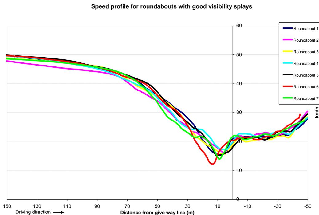
**FIGURE 8** Speed profiles for roundabouts with good visibility splays.
