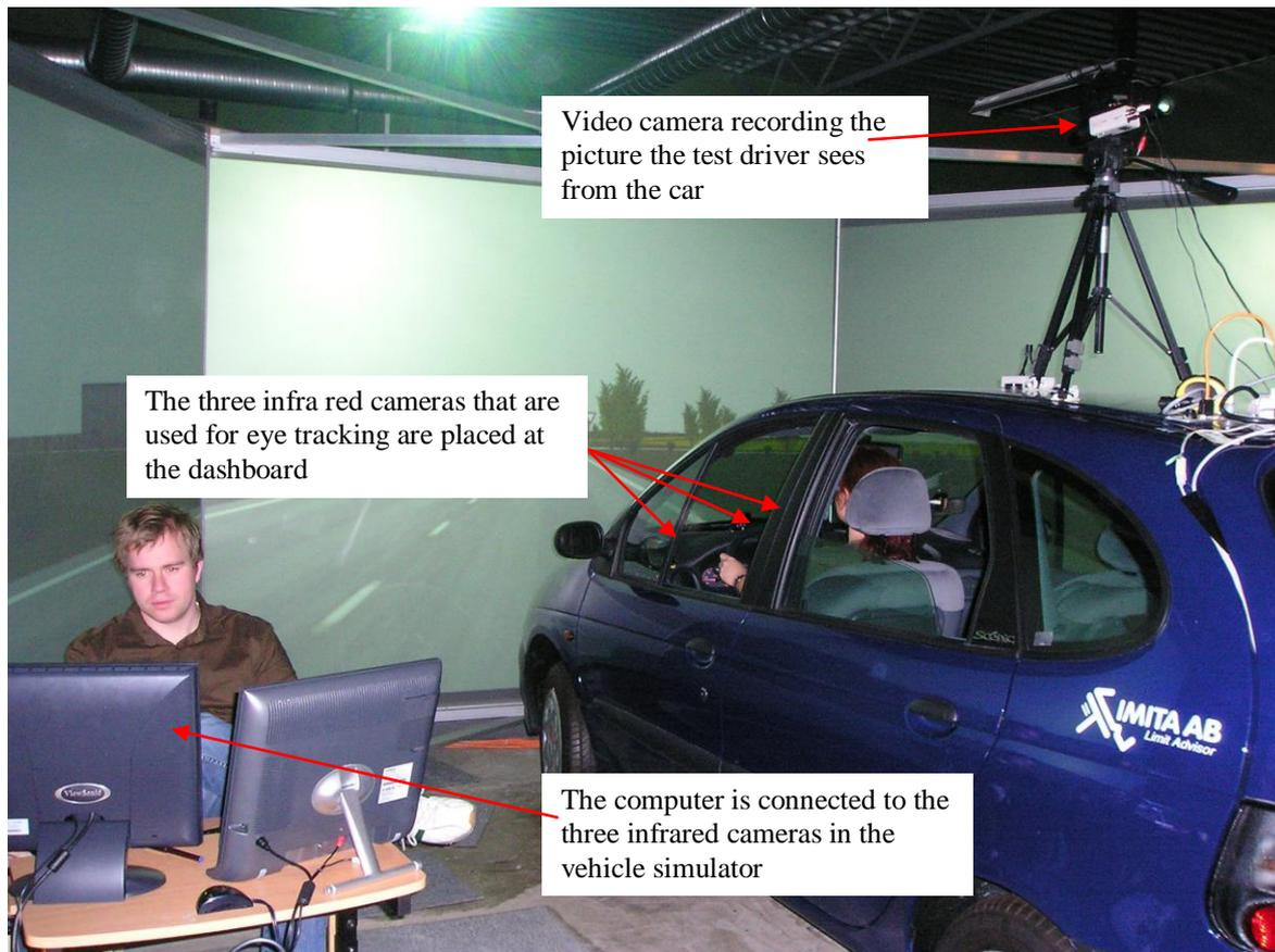
**FIGURE 3** The research set-up of eye tracking. The eye tracker consists of three infrared video cameras recording the face of the test driver during the test. The cameras are placed on the dashboard and connected to a computer, which amongst other things renders a computation of the test driver's visual focus.
