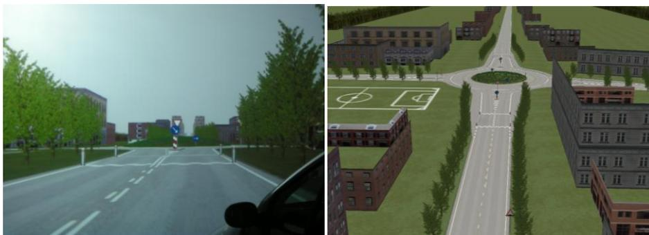
Example of roundabout with acceptable visibility splays. Height of the central island is 1.9 m with the plantation included. There are trees on the approach with an individual distance of 6 m.
