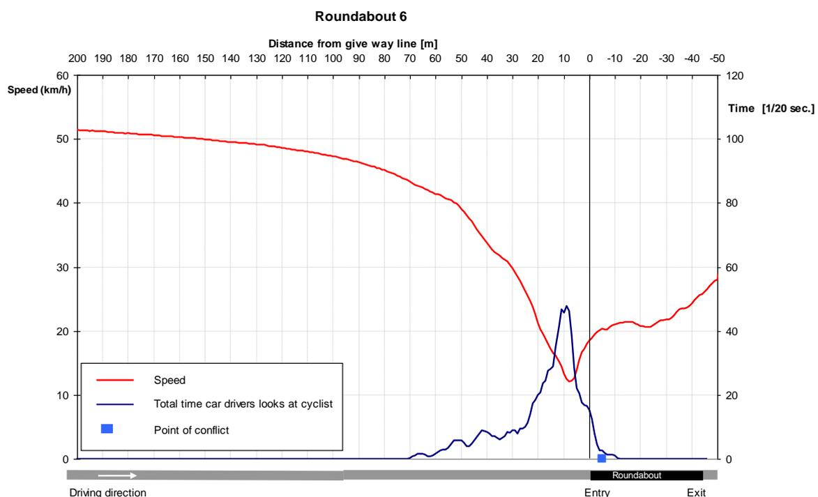
**FIGURE 9** Example of combined speed and glance profile for roundabout design 6. It clearly shows that the test drivers had the greatest visual focus on the cyclist at a distance of 10 meters from the give way line. The drivers' minimum speed on the approach is 12 km/h at a distance of 8 meters from the give way line.
