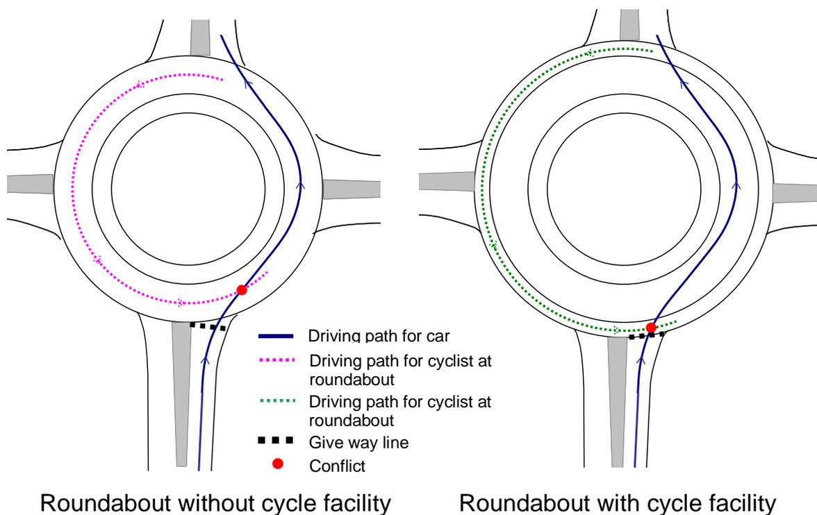
**FIGURE 6** Specification of driving paths for cyclists and cars, and indication of placement of conflict points and give way lines.
