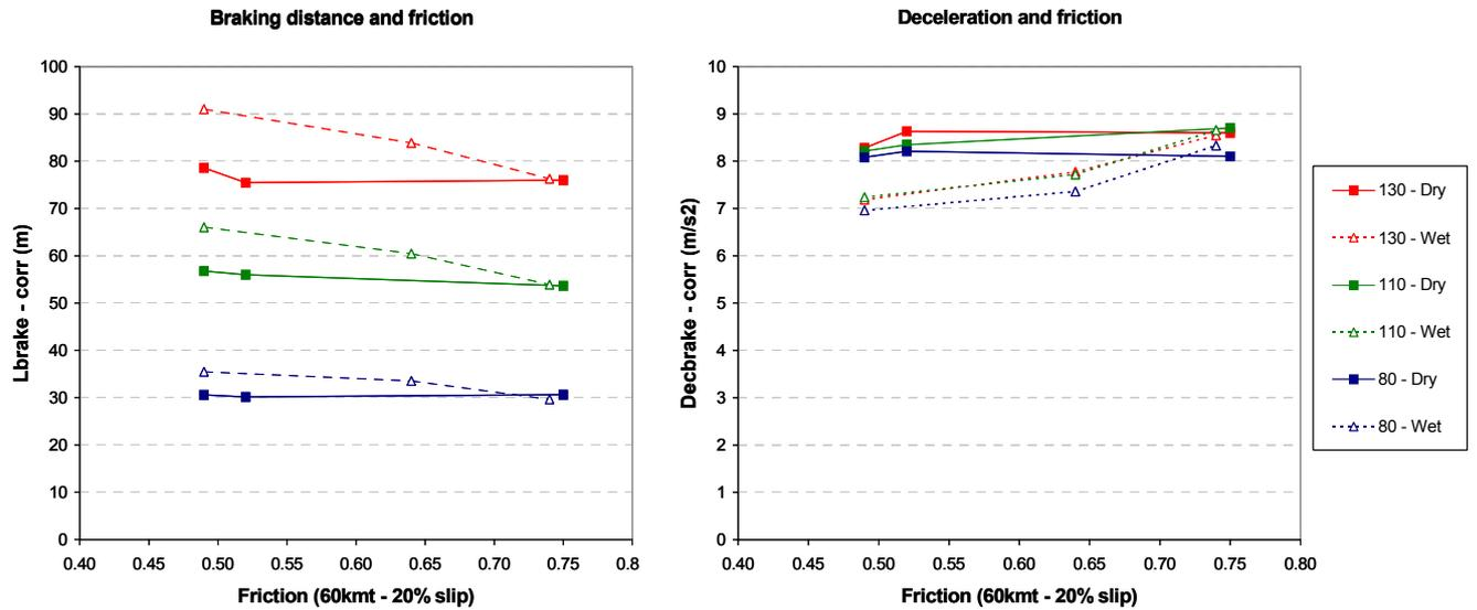
**FIGURE 2 Braking distance ( $L_{brake}$ ) and deceleration ( $Dec_{brake}$ ) as a function of friction.**
