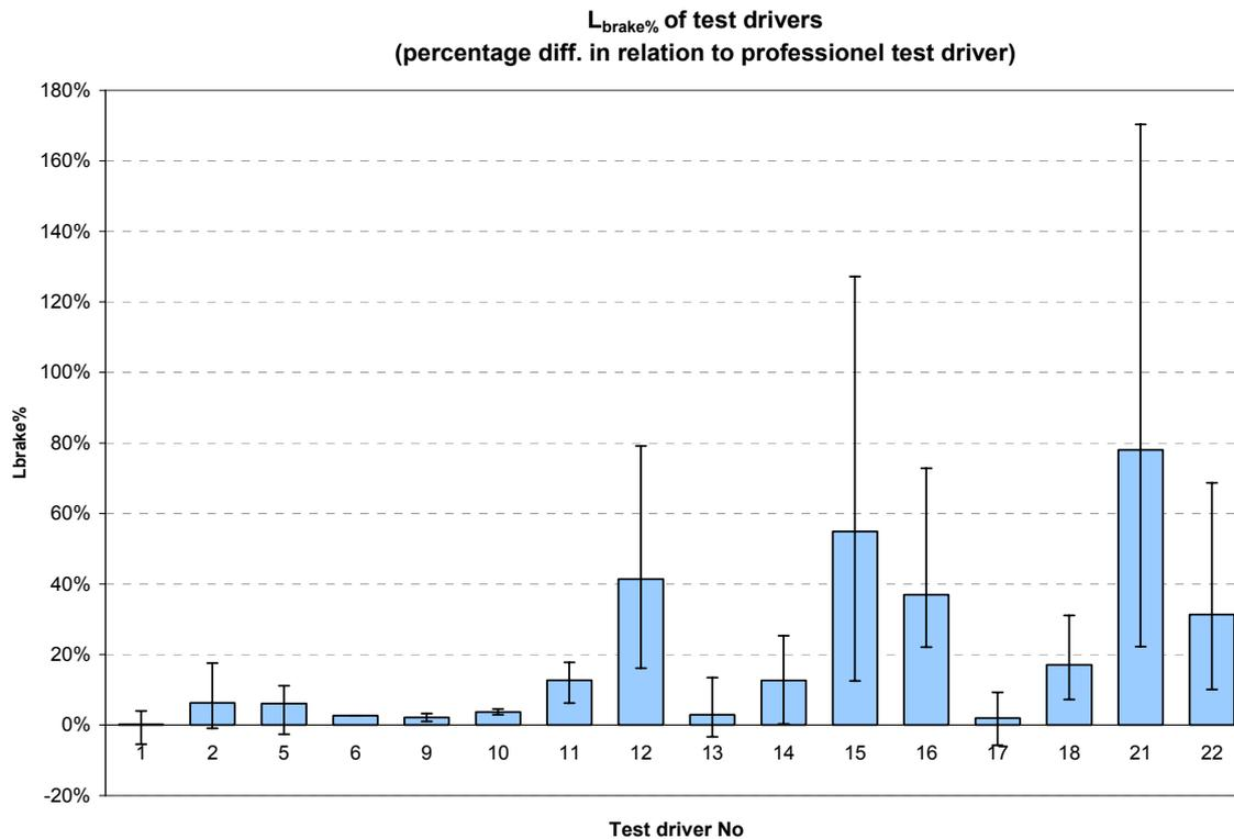
**FIGURE 3** L<sub>brake%</sub> for non professional test drivers, expressed as a mean, min. and max. value.
