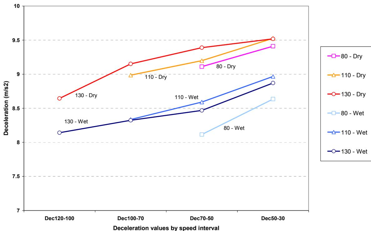
**FIGURE 1 Average deceleration values ( $\text{m/s}^2$ ) on dry and wet road, by speed intervals and initial speed.**
