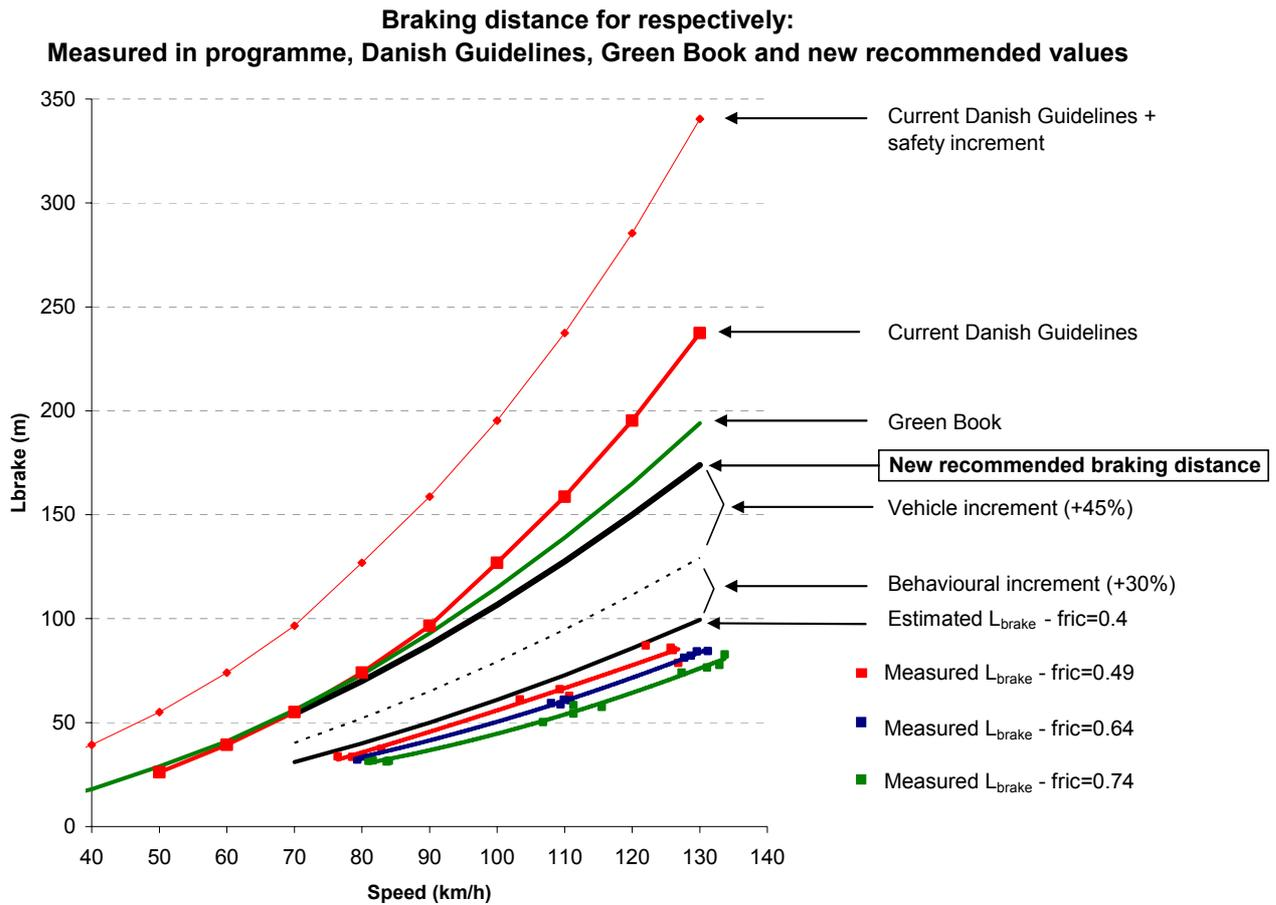
**FIGURE 4 Recorded values for  $L_{brake}$  and new and existing recommended braking distances**
