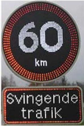
Figure 12: VMS sign showing temporary speed limit and warning for crossing traffic ahead.
