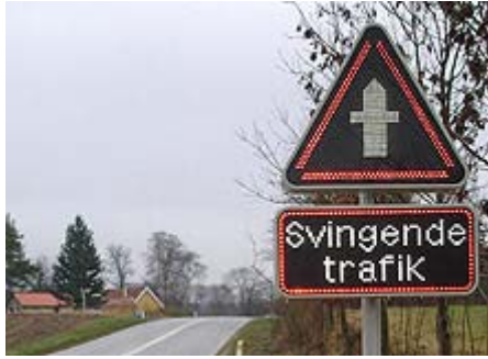
Figure 7.2: Warning sign showing crossing traffic in the intersection ahead
